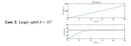
Disturbance attenuation: The same PI controller gives no steady-state error
