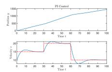
**Robustness**: The same PI controller can make the closed-loop system follow a reference signal even when some system parameters are not known exactly.
