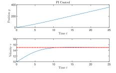
Disturbance attenuation: The same PI controller gives no steady-state error
