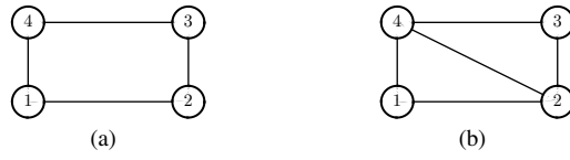
Fig. 1 (a) Nonchordal graph: the cycle (1-2-3-4) is of length four but has no chords. (b) Chordal graph: all cycles of length no less than four have a chord; the maximal cliques are \mathcal{C}_1 = \{1, 2, 4\} and \mathcal{C}_2 = \{2, 3, 4\} .
